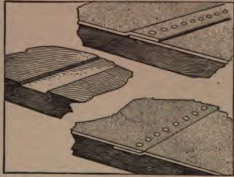
Porch Roofing, when Laid So as to Avoid Ridges Where the Strips Overlap, will Be Much More Durable
